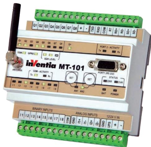
Telemetry Module MT-101 is a professional device combining functionality of programmable logic controller, data logger, protocol converter and wireless communication interface for GPRS packet transmission over GSM network. Compact, robust design, integral GSM modem, attractive technical features and easy to use configuration tools are important advantages of MT-101 in wireless, scalable, multinode systems for telemetry, control, diagnostic, surveillance and alarming.
