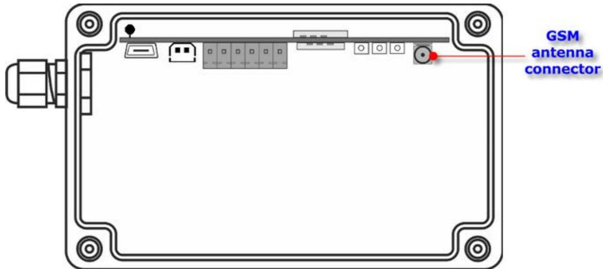
Depending on local signal propagation and user's needs different antenna types may be used. Proper antenna placement is important during the module installation. In case of low GSM signal level using the external directional antenna or high gain antenna may be necessary. On user request, MT-051 can be equipped with external antenna connector (SMA type).
