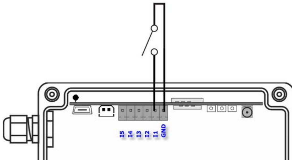
To maintain IP rating of the module, user shall ensure that connecting cable entering module is correctly secured and sealed by a cable gland. It is recommended to use cables with a circular cross-section. Usage of cables with different cross-section does not warrant maintaining tightness of the system.
