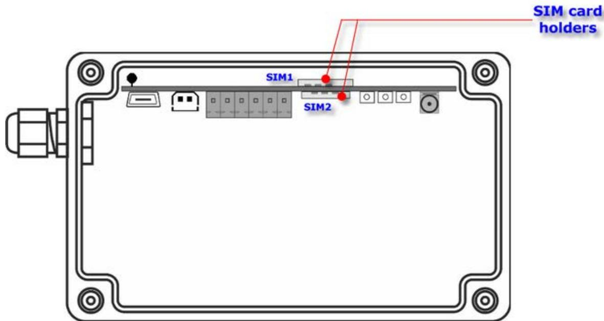
Proper insertion of the **SIM** card is essential for module's operation in GSM network. The module accepts only **SIM** cards in **3,3V** low voltage technology. For proper operation, at least one SIM card should be inserted into holder. If only one SIM card is used, it should be inserted in holder marked **SIM1**.
