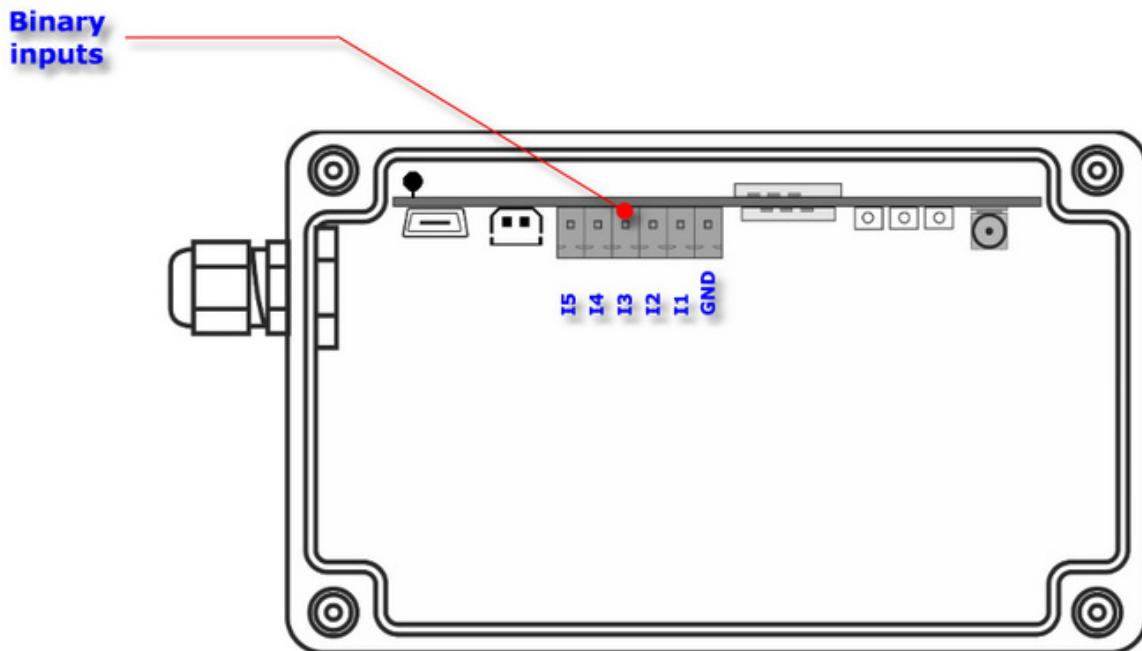
Inputs are designed to cooperate with potential free contacts (contacts connecting the input and common for all inputs ground). The inputs operate in **positive logic**, meaning the input is low when connected to ground and high if the circuit is open. The contacts are polarized with potential of 2,8V in high state. Binary inputs **are not isolated**.
