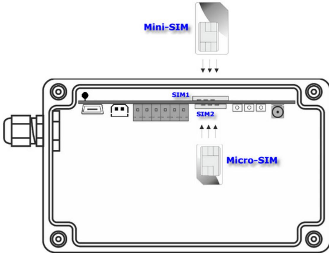
Correctly installed **SIM** cards secures connection between it's contact fields and the holder contacts.
