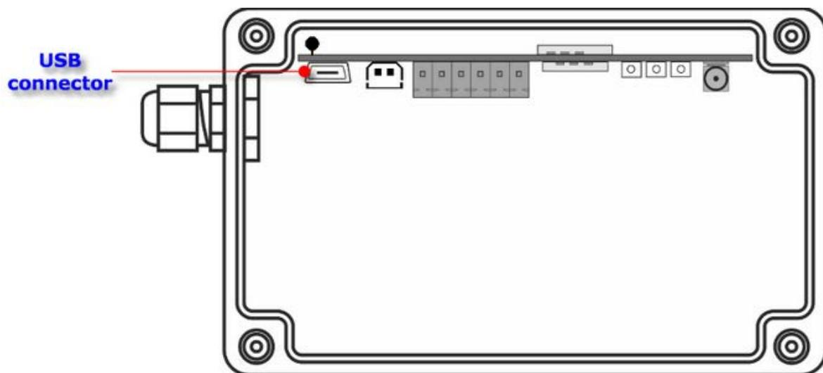
When module is connected via USB to a computer, it is powered via USB port. Thanks to that the module does not consume limited battery power during configuration and tests. During USB connection module does not enter power save mode.
