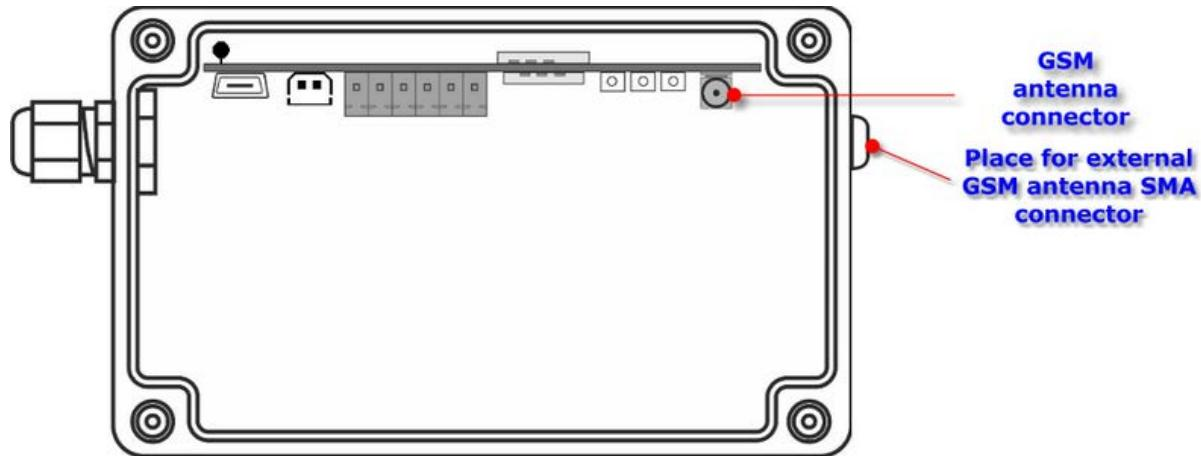
On user demand, module can be equipped with external SMA connector for GSM antenna - it will still maintain overall IP67 rating, but it is up to the user to secure antenna connector itself from water etc.
