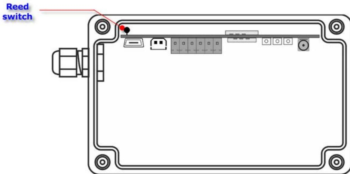
Activation of this input causes setting of **REED** flag and wakes module from sleep mode. Furthermore, activating reed switch for three times in several seconds intervals triggers GSM login procedure. This feature can be used to trigger events and/or during telemetry system tests.
