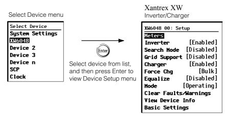
Figure 2-4 Selecting a Device Setup Menu
