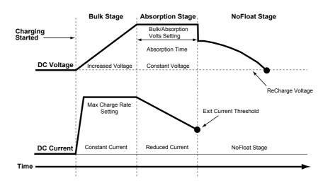
Figure 3-5 Two-Stage Charging Cycle
