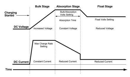
Figure 3-4 Three-Stage Battery Charging Cycle
