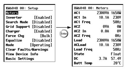
Figure 2-7 Viewing the Meters Screen
