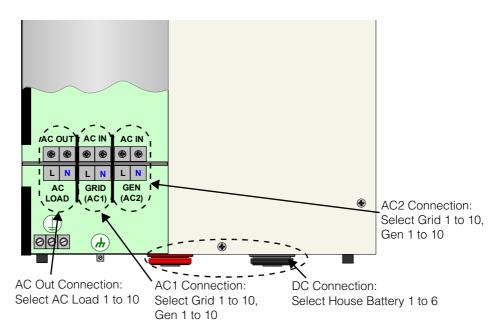
Figure 3-8 Xantrex XW Series Inverter/Charger Connections Representation
