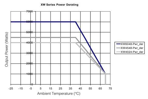
Figure A-2 Output Power Versus Ambient Temperature
