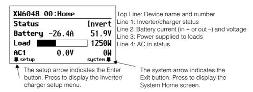
Figure 2-6 Xantrex XW Series Inverter/Charger Home Screen
