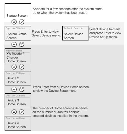
Figure 2-3 Xantrex XW System Control Panel Top Level Screens
