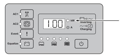
Figure 2-2 Inverter Information Panel When Inverting
