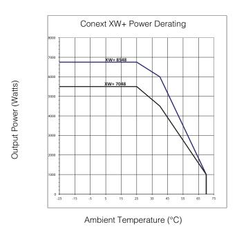
Figure A-2 Output Power Versus Ambient Temperature
