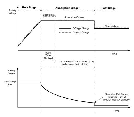
Figure 3-4 Three-Stage Battery Charging Cycle
