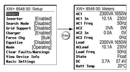
Figure 2-8 Viewing the Meters Screen
