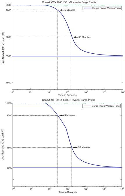
Figure A-1 Conext XW+ AC Overload Capability
