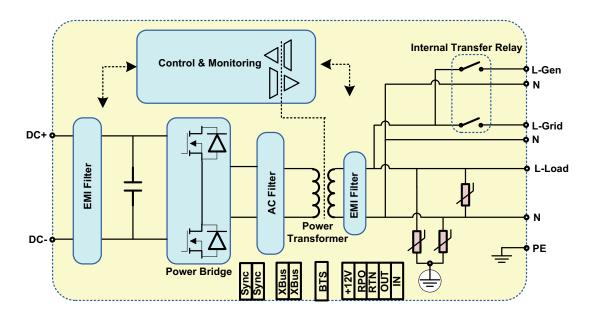
Figure A-6 Conext XW+ Block Diagram
