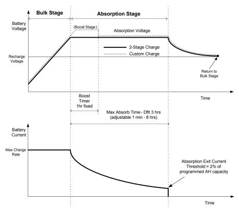
Figure 3-5 Two-Stage Charging Cycle
