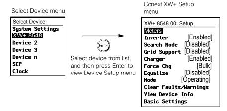
Figure 2-5 Selecting a Device Setup Menu
