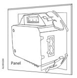
Fig.2-6 Use clips to fix the meter
