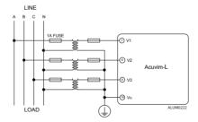
Fig.2-13b 3LN connection with 3PTs
