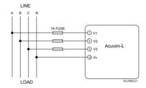
Fig.2-13a 3LN direct connection
