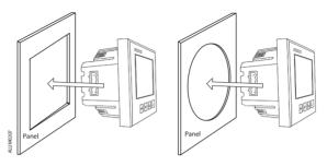
Fig.2-5 Put the meter into the square
