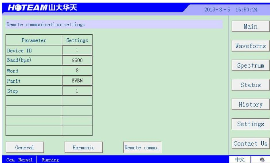
Fig.27: Remote communication customer settings
