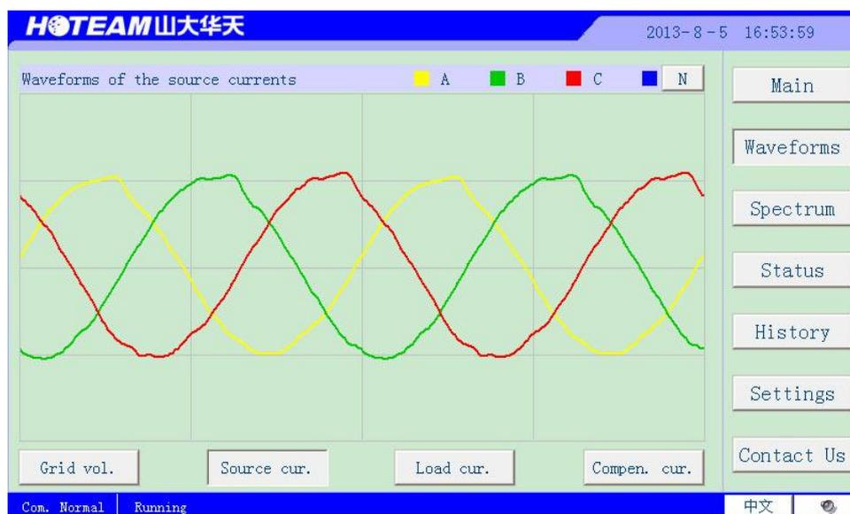
Fig.16: Source current waveforms
