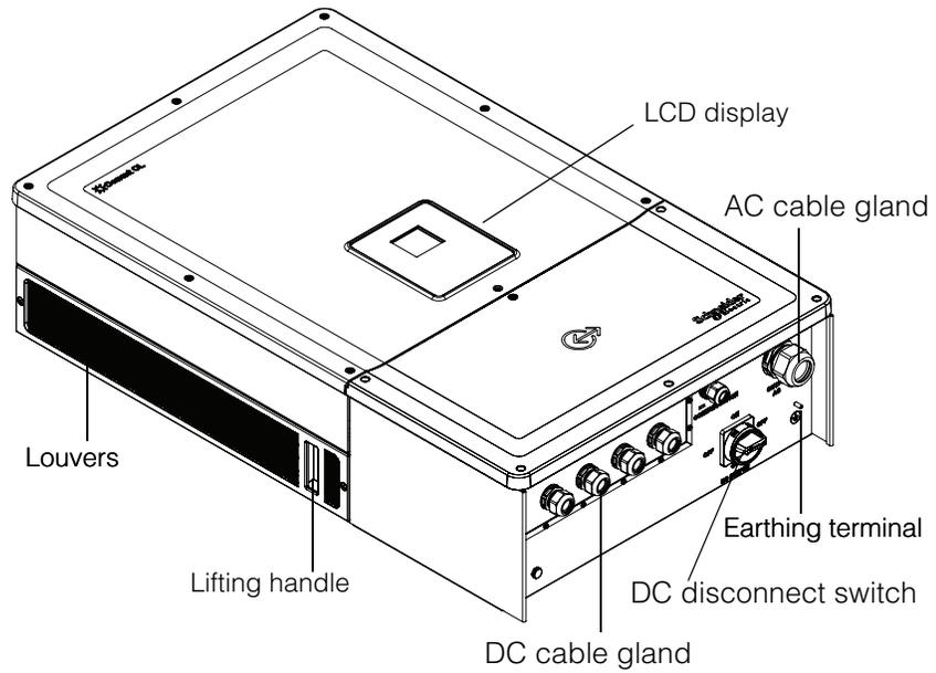
**Figure 1-4** Location of physical features of the inverter and the wiring box- left side view
