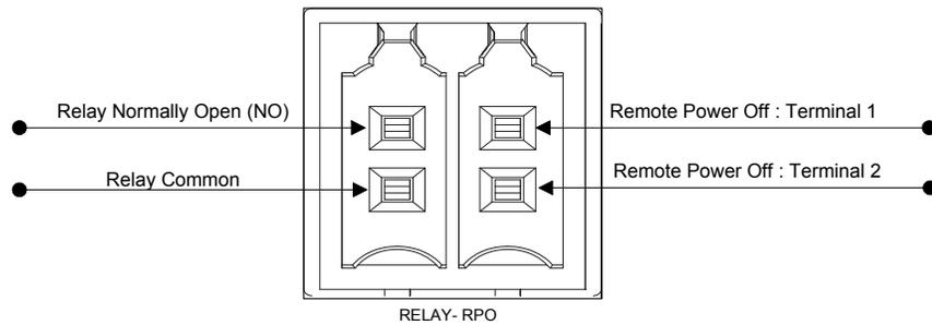
**Figure 2-48** RPO and Relay Contact terminal details
