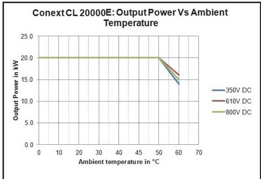
Figure A-3 Derating curve- 20KW
