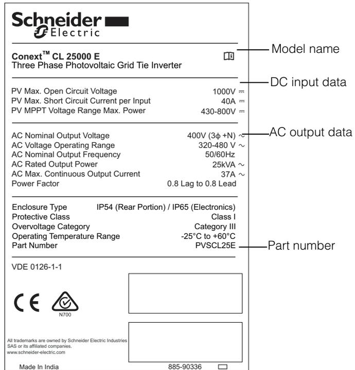
**Figure 2-4** Inverter nameplate label
