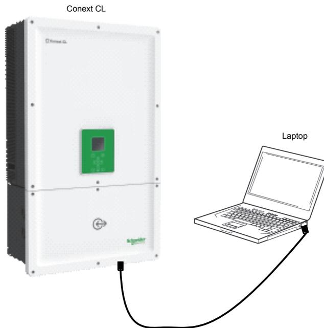
**Figure 2-55** Web interface connection diagram
