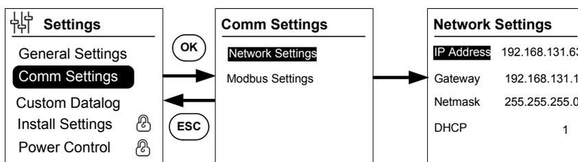
**Figure 2-54** Checking the IP address
