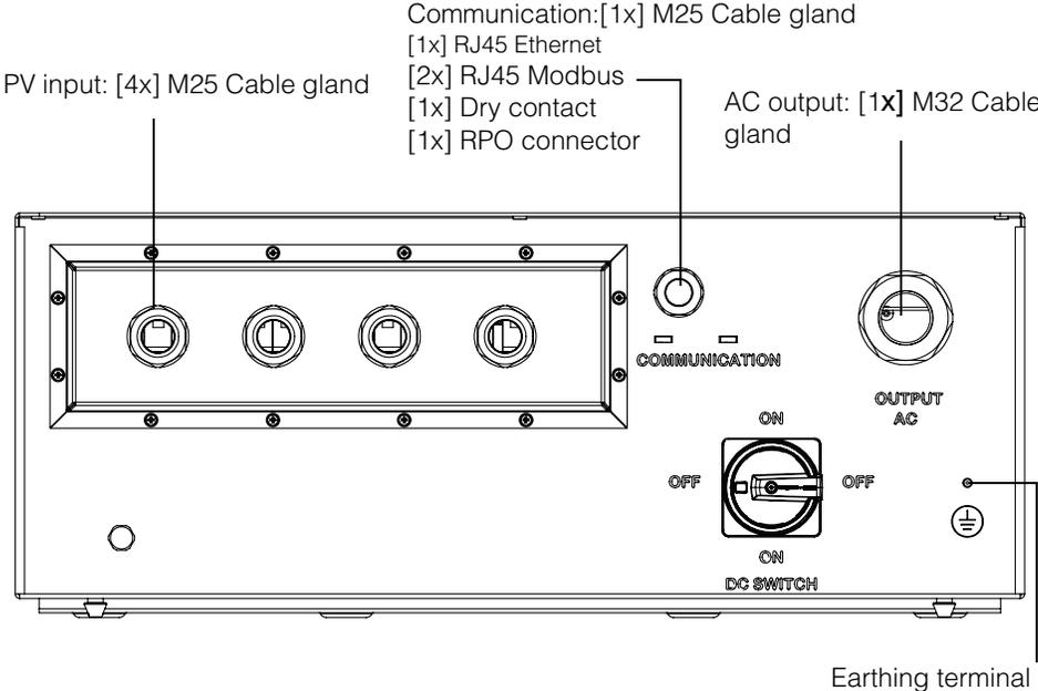
Figure 1-6 Bottom view of the wiring box
