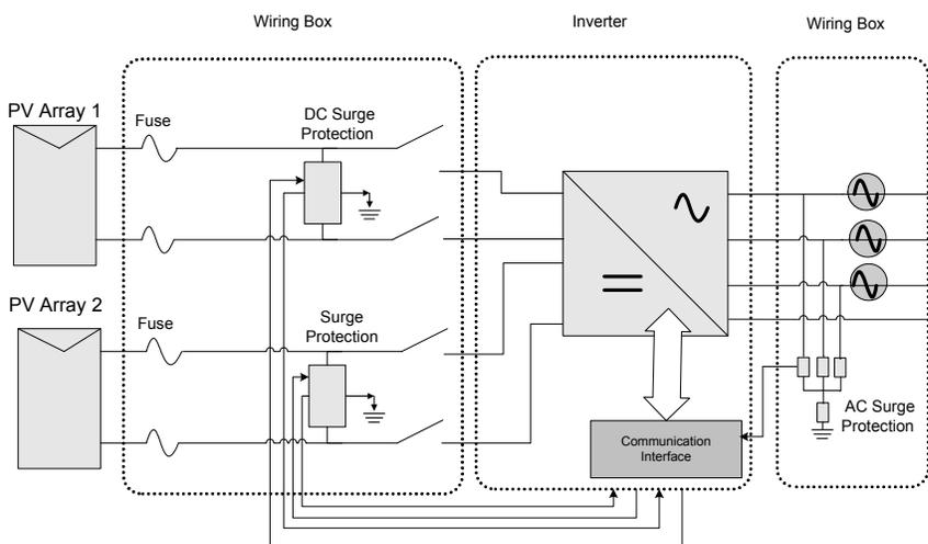
**Figure 2-53** Surge Protection device wiring
