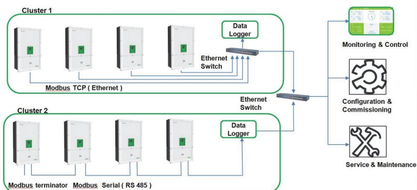
Figure 2-47 Cluster 1: Modbus TCP and Cluster 2: Modbus RS485 connections
