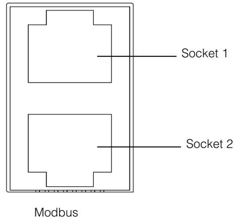
**Figure 2-44** Modbus (RS485) connectors
