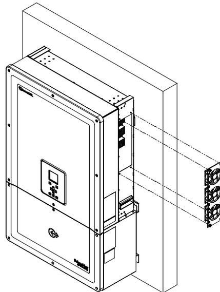
**Figure 5-6** Removing the fan
