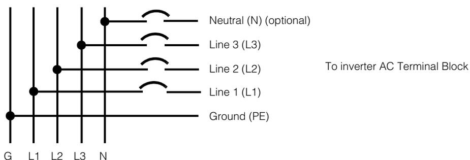
**Figure 2-38** AC connection details
