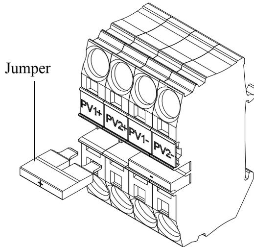
**Figure 2-34** MPPT Shorting Connector and Jumper arrangement
