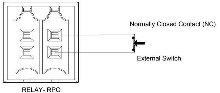
**Figure 2-51** RPO connection for single inverter
