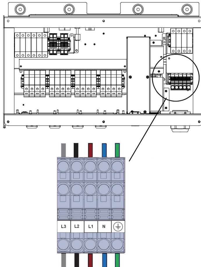
**Figure 2-36** Wire installation
