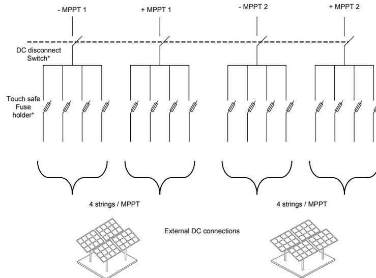
**Figure 2-33** PV Wiring diagram of the Conext CL 20000E and 25000E models
