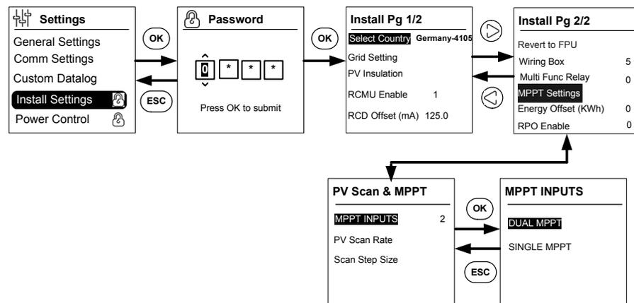
**Figure 2-35** MPPT settings through Install settings menu
