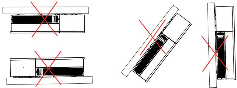
**Figure 2-7** Incorrect mounting positions
