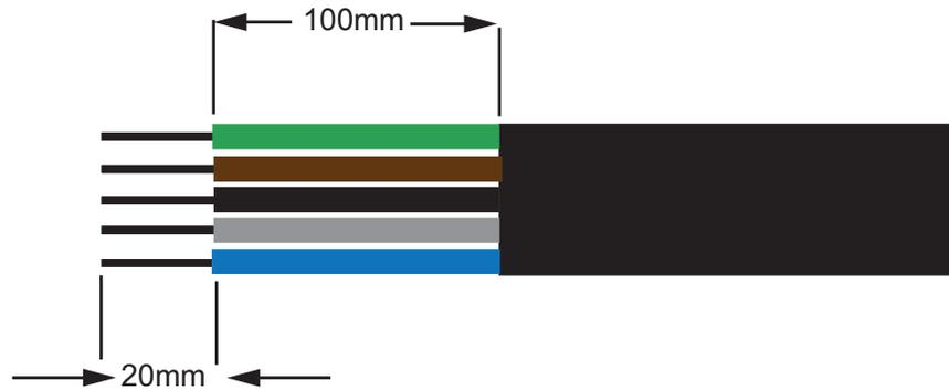
**Figure 2-39** AC wiring
