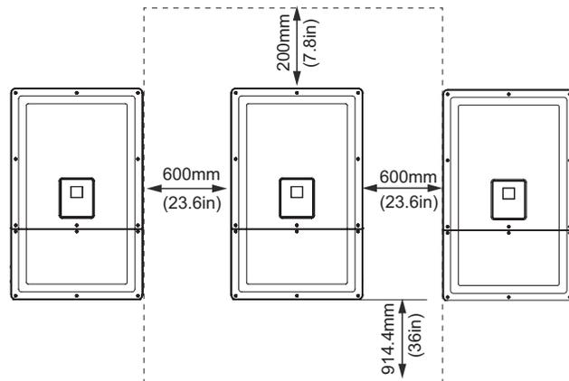
**Figure 2-8** Proper installation distances of the inverter
