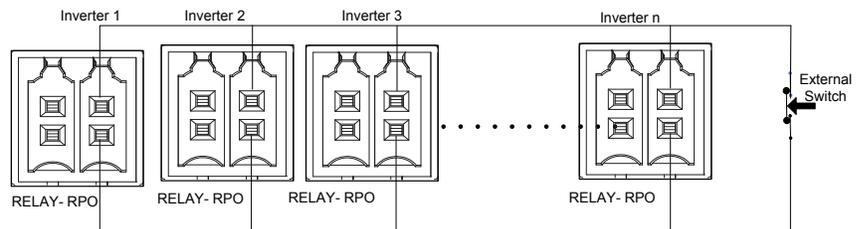
**Figure 2-52** RPO connection with multiple inverters
