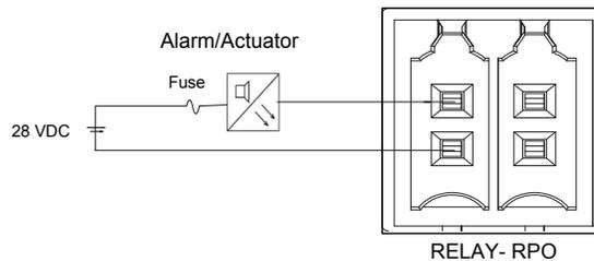
**Figure 2-49** Dry Contact Relay connection
