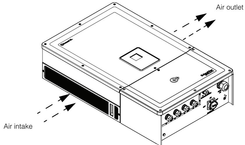
**Figure 1-5** Cooling arrangement of the inverter
