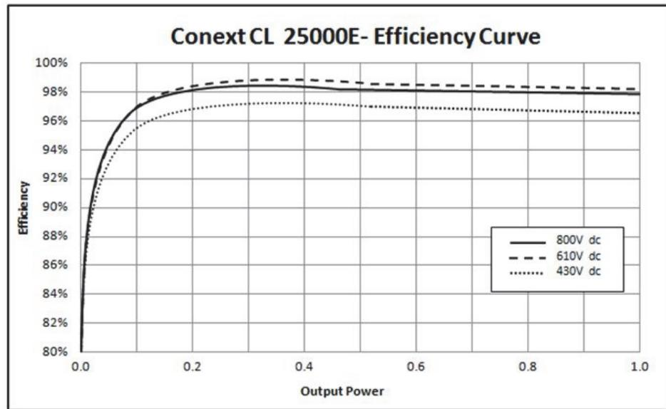
Figure A-2 Efficiency curve- 25KW
