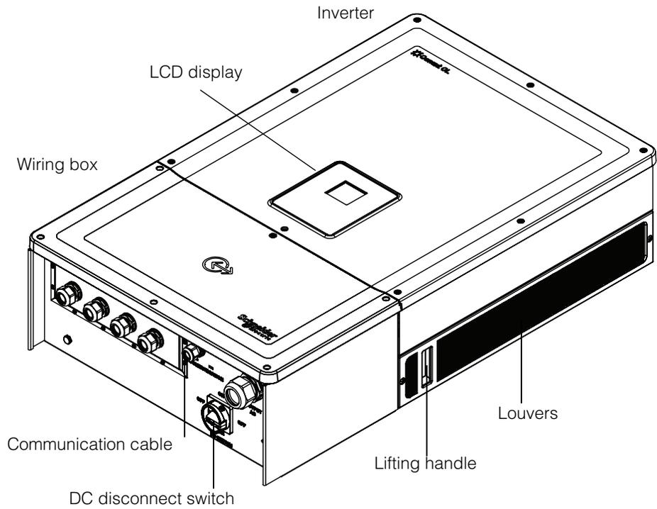
**Figure 1-3** Location of physical features of the inverter and the wiring box- right side view
