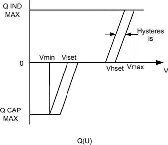
**Figure 3-18** Reactive power as a function of voltage
