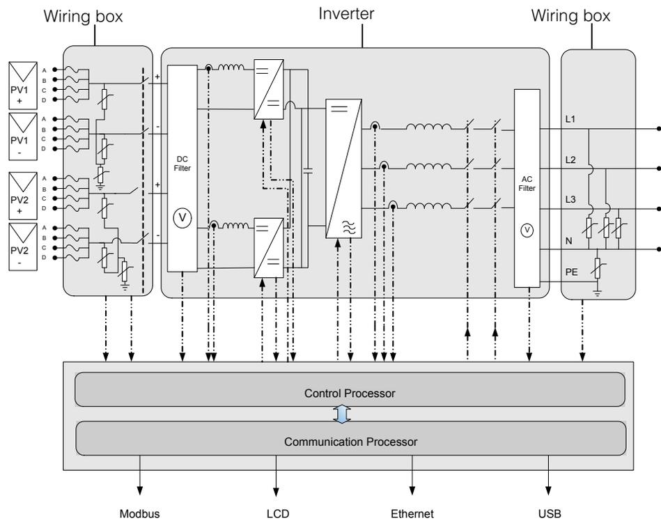
**Figure 1-2** Block diagram of the Conext CL 20000E and 25000E models
