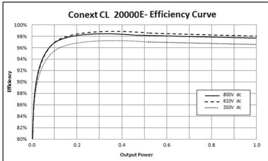
Figure A-1 Efficiency curve - 20KW
