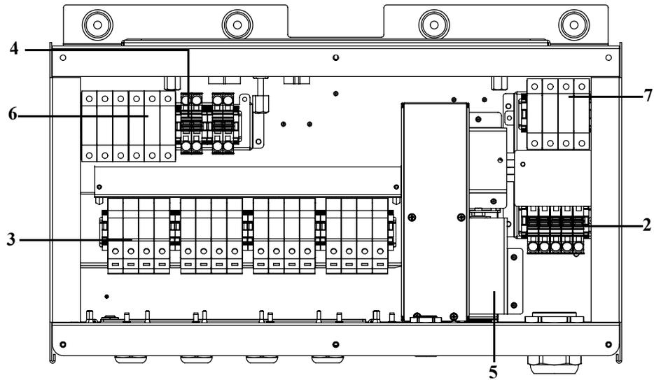
**Figure 2-13** Wiring box- Optimum (PVSC2025E300)
