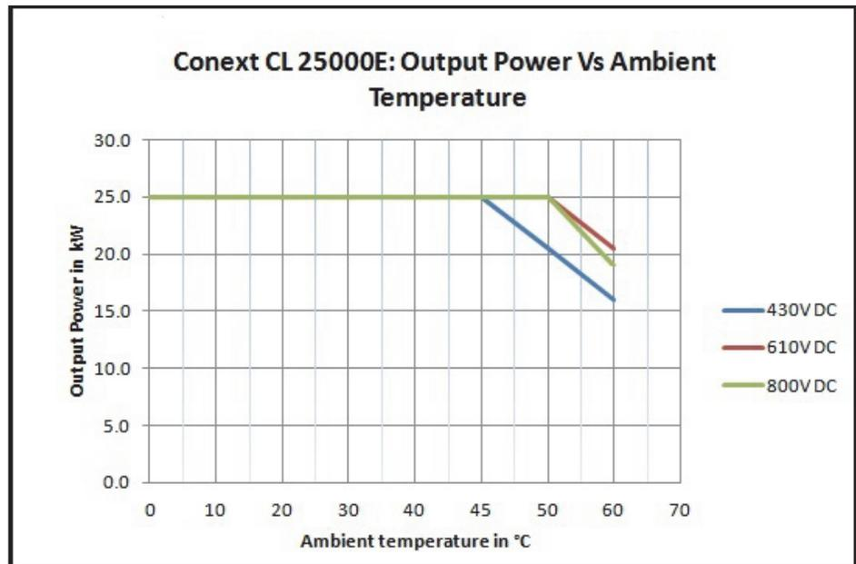
Figure A-4 Derating curve- 25KW
