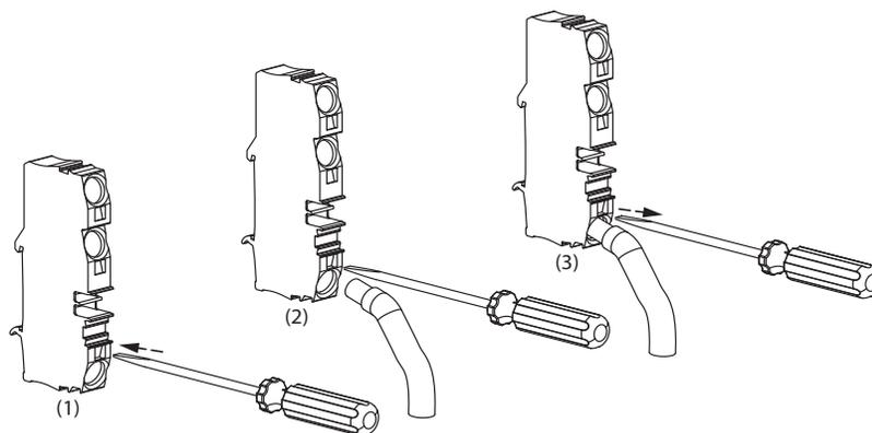
**Figure 2-37** Wire installation
