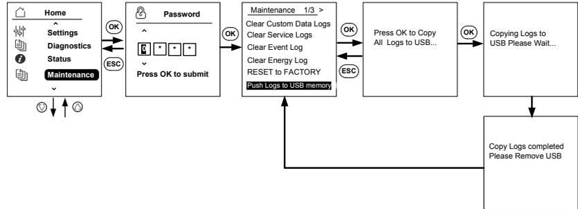
Figure 5-16 Pushing logs to USB
