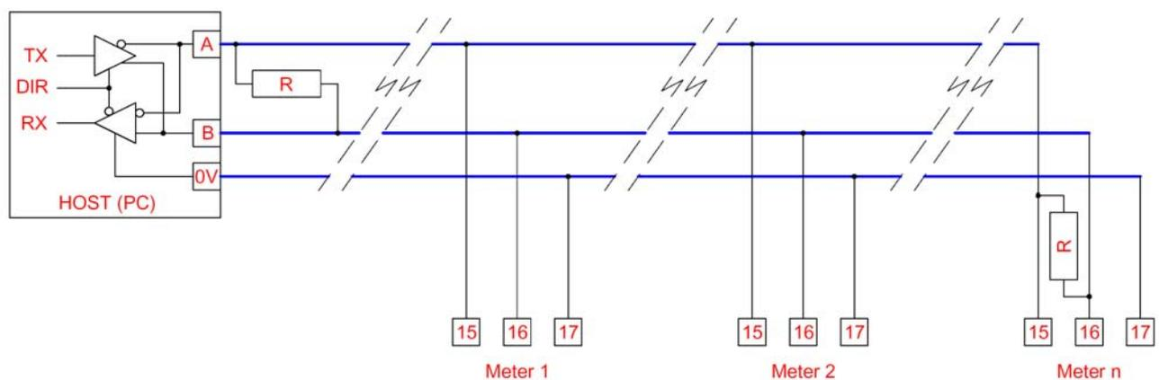
Figure 3-1 Basic RS485 Bus Network
