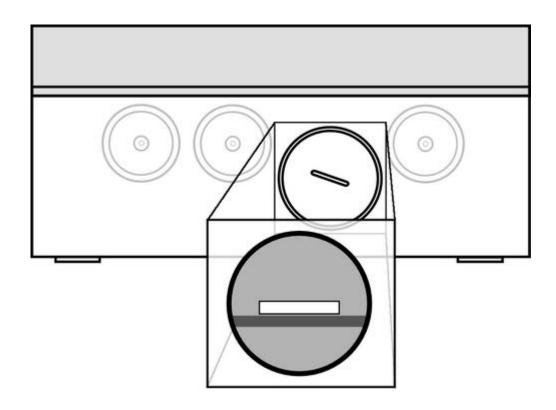
Proper insertion of the **SIM** card is essential for module's operation in GSM network. The module accepts only **SIM** cards in **3,3V** low voltage technology.
