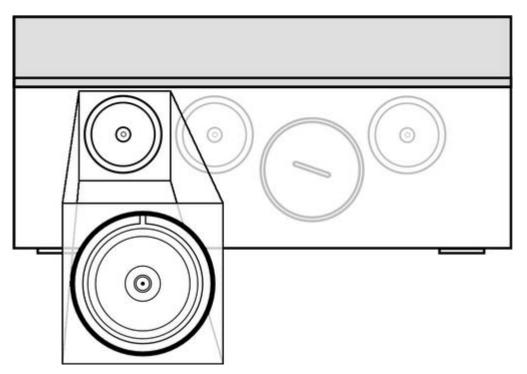
Connection between plug and socket should be secured with locking ring to ensure certainty of the connection. Unused slots should be secured with protective caps.
