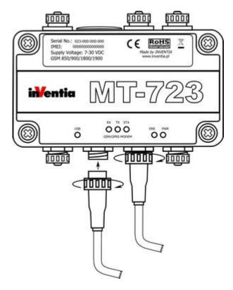
Connection between plug and socket should be secured with locking ring to ensure certainty of the connection. Unused slots should be secured with protective caps. Assembly of IP68 plug is described in the instruction attached to the elements of the plug. It is recommended to use cables with a circular cross-section. Usage of cables with different cross-section does not warrant maintaining tightness of the system.
