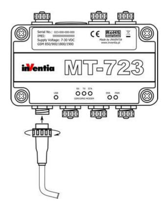
Assembly of IP68 plug is described in the instruction attached to the elements of the plug. It is recommended to use cables with a circular cross-section. Usage of cables with different cross-section does not warrant maintaining tightness of the system.
