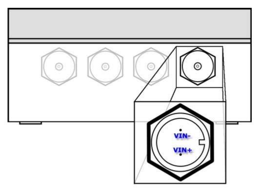
It is recommended to place the power supply in IP68 enclosure and ensure the connection with module is of the same class. Any power source housing or connectors leakage may allow water penetration and consequently damage electronic components of module. Proper power source connection is described in <u>Power supply</u> subchapter of <u>Connection diagrams</u> chapter.
