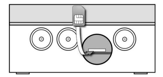
Correctly installed **SIM** card secures connection between its contact fields and the holder contacts.
