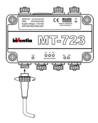
Assembly of IP68 plug is described in the instruction attached to the elements of the plug. It is recommended to use cables with a circular cross-section. Usage of cables with different cross-section does not warrant maintaining tightness of the system.
