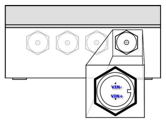
It is recommended to place the power supply in IP68 enclosure and ensure the connection with module is of the same class. Any power source housing or connectors leakage may allow water penetration and consequently damage electronic components of module. Proper power source connection is described in <u>Power supply</u> subchapter of <u>Connection diagrams chapter</u>.
