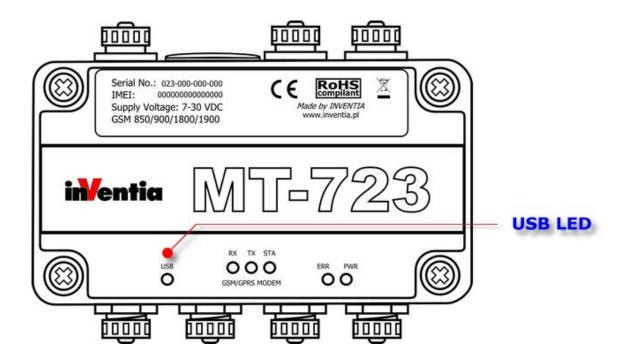
Detailed information on using the **USB** port for module configuration can be found in the **MTManager2.0** manual.
