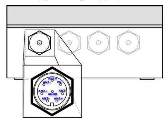
The inputs are designed to work with analog sensors generating signal in 0...5V range. In order to minimize energy consumption the A/C converters are powered for the period necessary to conduct secure measurement.
