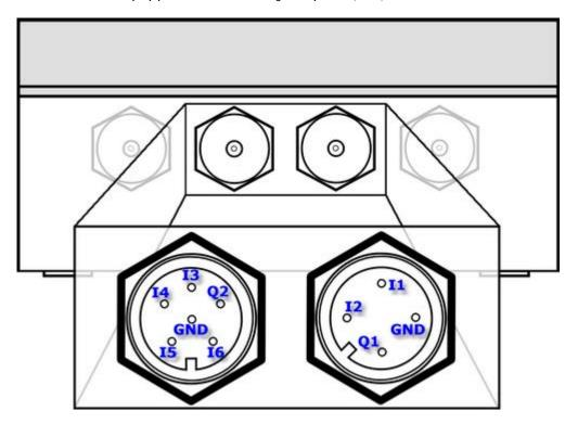
The outputs are designed to control loads powered by internal source (e.g. light signaling). The outputs are of "open drain" type controlled by NMOS transistors. In High state the output is shorted to the ground by active NMOS transistor. In case of inductive type load connected (a relay) the circuit limiting voltage peaks to max. +30V is necessary.
