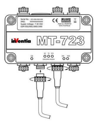
Connection between plug and socket should be secured with locking ring to ensure certainty of the connection. Unused slots should be secured with protective caps. Assembly of IP68 plug is described in the instruction attached to the elements of the plug. It is recommended to use cables with a circular cross-section. Usage of cables with different cross-section does not warrant maintaining tightness of the system.
