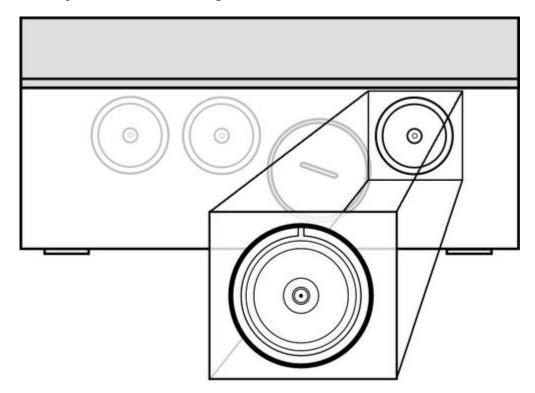
Connection between plug and socket should be secured with locking ring to ensure certainty of the connection. Unused slots should be secured with protective caps.
