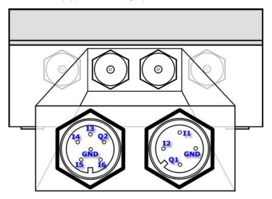
Inputs **I1...I6** are designed to cooperate with potential free contacts (contacts connecting the input and common for all inputs ground). The inputs operate in **negative logic**, meaning the input is high when connected to ground and low if the circuit is open. This solution allows energy saving, a crucial ability for battery driven devices. The contacts are polarized with potential of 3V in low state. Binary inputs **are not isolated.**
