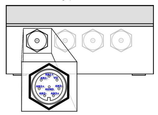
This output allows user to power sensors with voltage ranging from **0** to **5VDC** with step **0.1V**. Voltage is specified by the user parameter configuration.
