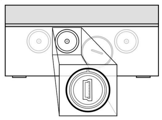
When module is connected via USB to a computer, it is powered via USB port. Thanks to that the module does not consume limited battery power during configuration and tests. During USB connection **VBAT** register holding data of battery voltage is **frozen on the last recorded value** (at first configuration the value is 0).
