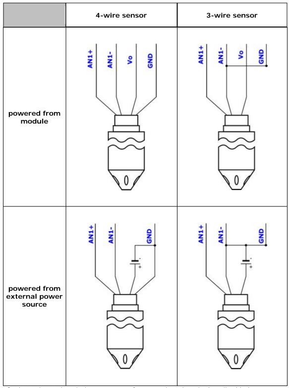
Sockets pinout description necessary for preparing plugs is described below:
