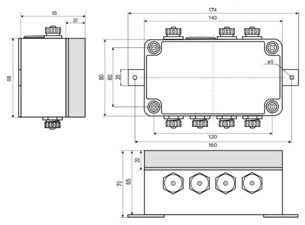
Please note that the degree of protection is highly dependent on used connectors. Connectors used in the construction ensure maintaining IP68 protection degree. **Using other connectors may result in water penetration and consequently cause device damage.**
