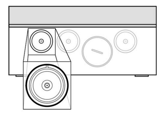
Depending on local signal propagation and user's needs different antenna types may be used. Proper antenna placement is important during the module installation. In case of low GSM signal level using the directional antenna or antenna high gain may be necessary.
