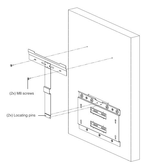
Figure 2-17 Fastening the inverter mounting plate to the wall
