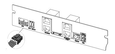
Figure 2-43 SPD monitoring cable connection
