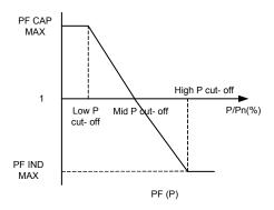
Figure 3-17 Active power as a function of power factor
