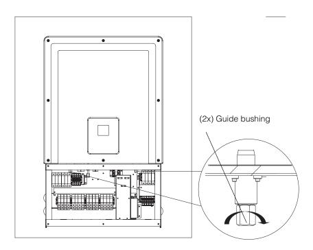
Figure 2-30 Locking the inverter to the wiring box
