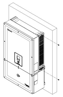
Figure 5-1 Loosening the louver cover- right side
