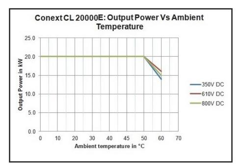
Figure A-3 Derating curve- 20KW
