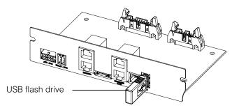
Figure 5-10 Communication interface with USB flash drive
