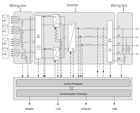
Figure 1-2 Block diagram of the Conext CL 20000E and 25000E models
