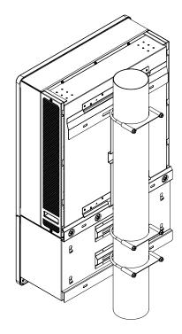
Figure 2-21 Pole mounting- rear view with the inverter installed
