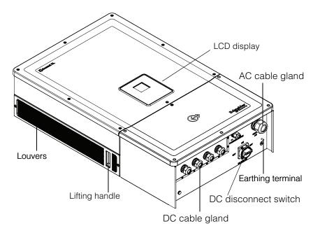
Figure 1-4 Location of physical features of the inverter and the wiring box- left side view
