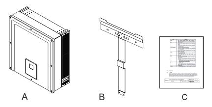
Figure 2-3 Packing list- Inverter
