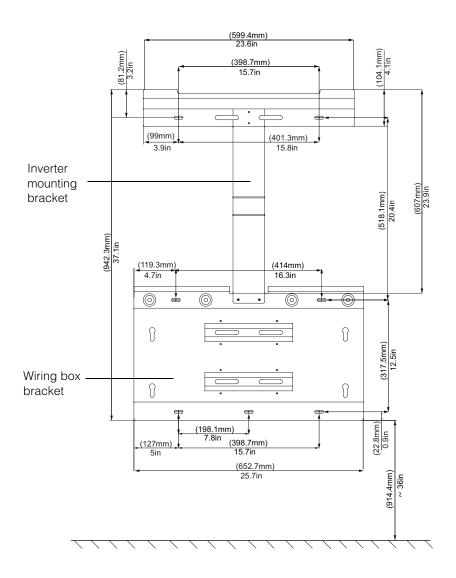
Figure 2-15 Mounting bracket dimensions- Wiring box and Inverter
