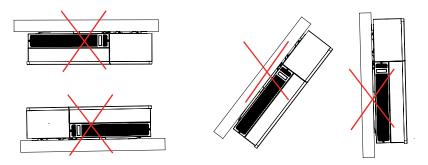
Figure 2-7 Incorrect mounting positions
