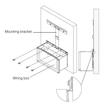
Figure 2-24 Fastening the wiring box to the mounting bracket
