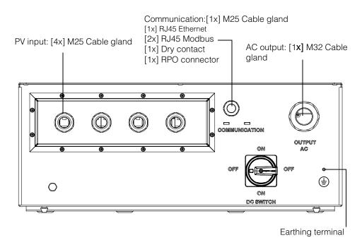
The Ingress Protection rated cable glands/ pv connectors are located at the bottom of the wiring box, as shown in Figure 1-6.
