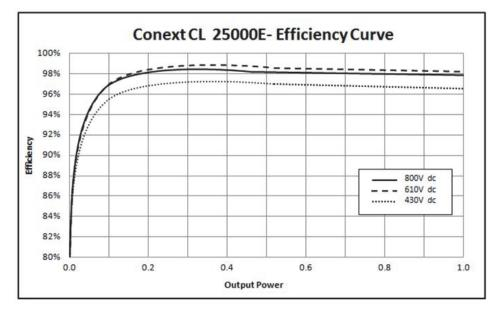
Figure A-2 Efficiency curve- 25KW
