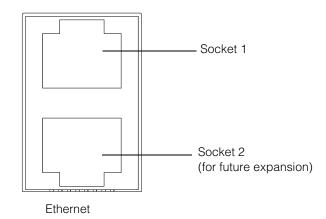
Figure 2-45 Ethernet Connection
