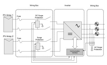
Figure 2-53 Surge Protection device wiring
