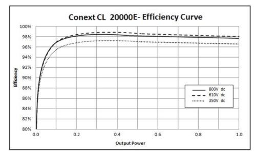
Figure A-1 Efficiency curve - 20KW
