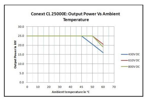
Figure A-4 Derating curve- 25KW
