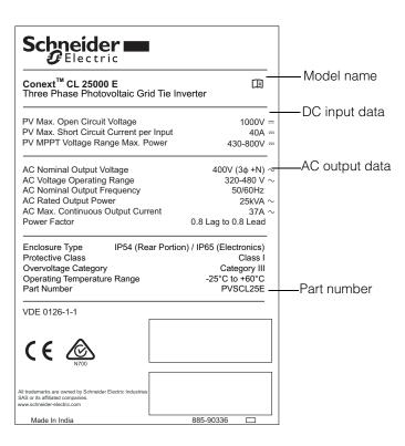
Figure 2-4 Inverter nameplate label
