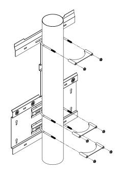
Figure 2-20 Rear view of the pole mounting installation
