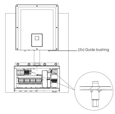
Figure 2-29 Inverter assembly- front view
