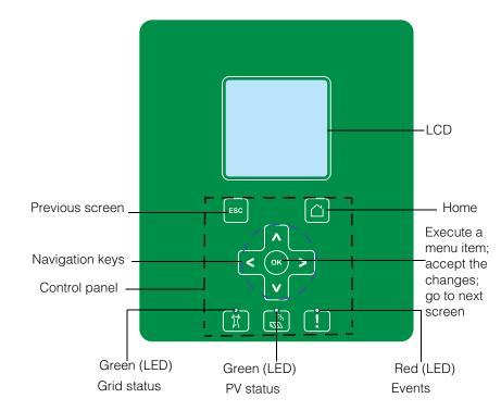
Figure 3-1 LCD Control Panel
