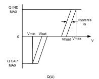
Figure 3-18 Reactive power as a function of voltage
