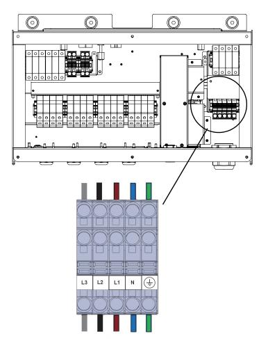
Figure 2-36 Wire installation
