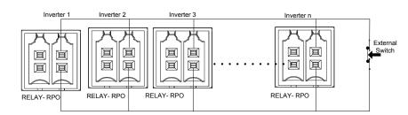
Figure 2-52 RPO connection with multiple inverters
