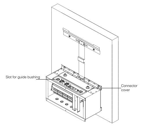
Figure 2-27 Anchoring the connector cover
