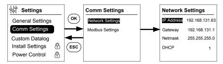
Figure 2-54 Checking the IP address
