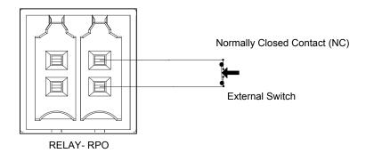
Figure 2-51 RPO connection for single inverter
