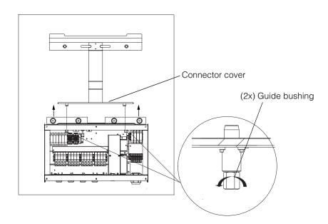
Figure 2-26 Removing the connector cover
