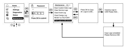
Figure 5-16 Pushing logs to USB
