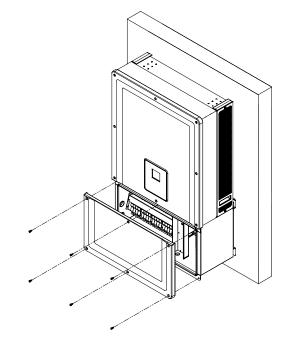
Figure 2-32 Closing the wiring box
