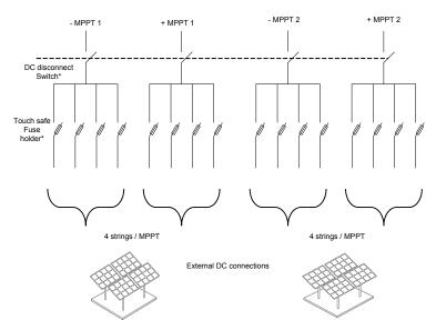
The inverter can accept PV input on all the four PV array input terminals on each MPPT. A maximum of four PV string inputs can be connected to each MPPT.
