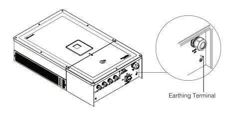
Figure 2-40 Connecting the earthing conductor
