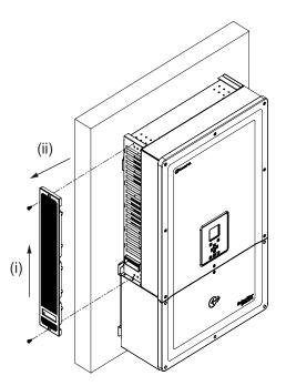
Figure 5-4 Removing the louver cover- left side
