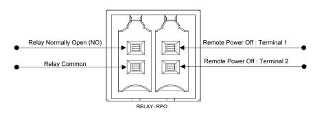
Figure 2-48 RPO and Relay Contact terminal details
