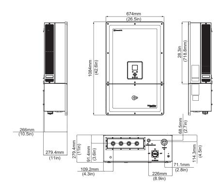
Figure 2-9 Views and dimensions of the inverter and the wiring box (Essential/ Optimum)
