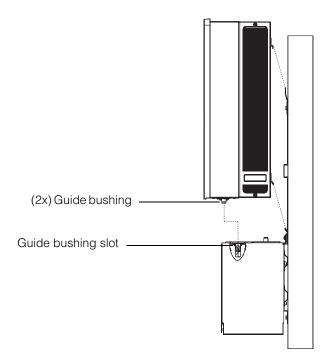
Figure 2-28 Inverter assembly- side view
