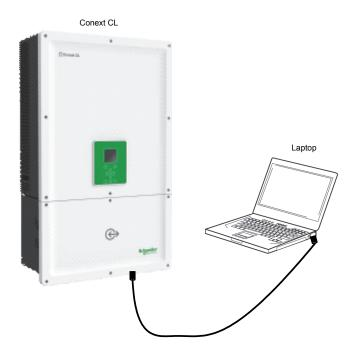
Figure 2-55 Web interface connection diagram
