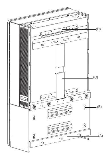
Figure 2-18 Inverter rear view with mounting bracket
