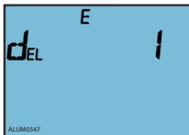
Fig.3-50 Clear energy enable setting
