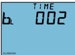
Fig.3-47 Backlight "ON" time setting
