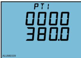
Fig.3-42 PT primary side ratio setting
