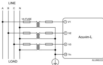
Fig.2-13b 3LN connection with 3PTs
