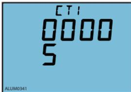
Fig.3-44 CT primary side ratio setting
