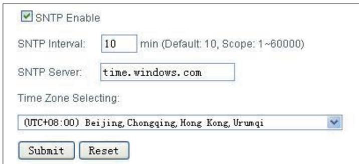
The screenshot shows a web-based configuration interface for SNTP settings. At the top, there is a checkbox labeled "SNTP Enable" which is checked. Below this, the "SNTP Interval" is set to "10" minutes, with a note "(Default: 10, Scope: 1~60000)". The "SNTP Server" is set to "time.windows.com". Under "Time Zone Selecting:", a dropdown menu is open, showing the selected option "(UTC+08:00) Beijing, Chongqing, Hong Kong, Urumqi". At the bottom of the form are two buttons: "Submit" and "Reset".
