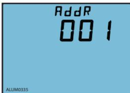
Fig.3-37 Communication address setting
