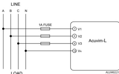
Fig.2-13a 3LN direct connection
