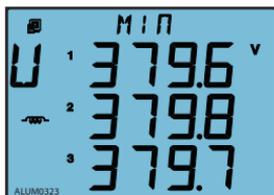
Fig.3-25 Min value of phase voltage
