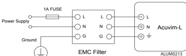
Fig.2-12 wiring connection of auxiliary power supply with EMC filters
