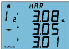
Fig.3-35 2<sup>nd</sup> harmonic content of current
