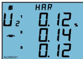
Fig.3-33 2<sup>nd</sup> harmonic content of phase voltage
