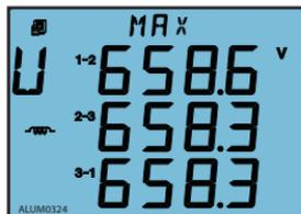
Fig.3-26 Max value of line to line voltage
