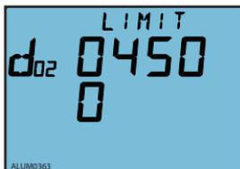
Fig.3-70 DO2 alarm limit setting
