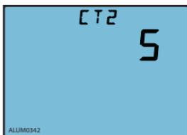
Fig.3-45 CT secondary side ratio setting
