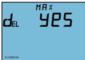
Fig.3-49 Clear Max and Min page setting
