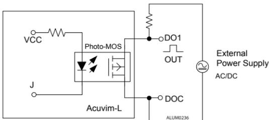
Fig.2-27 Digital output circuit
