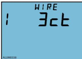
Fig.3-41 Current input wiring setting
