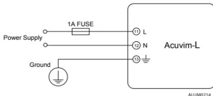
Fig.2-11 wiring connection of power supply
