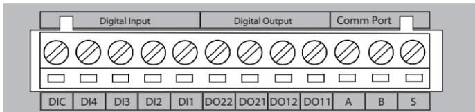
Fig.2-9 Expansion module terminal description
