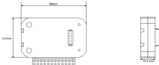
Fig.2-2 structure configuration of IO modules
