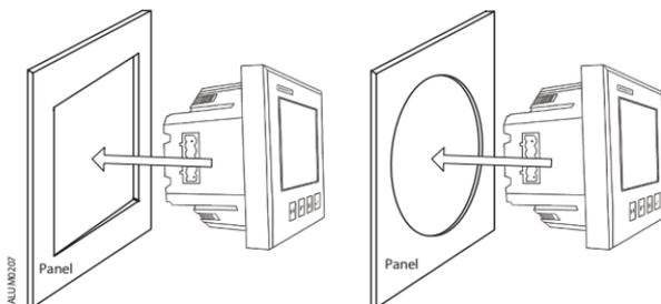
Fig.2-5 Put the meter into the square
