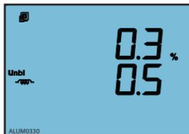
Fig.3-32 Unbalance factor for voltage and current
