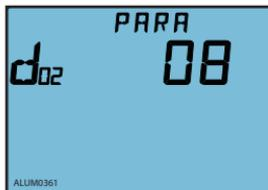
Fig.3-68 DO2 alarm output item setting
