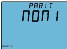
Fig.3-57 Extend IO communication check setting
