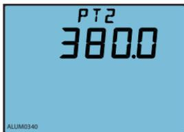
Fig.3-43 PT secondary side ratio setting
