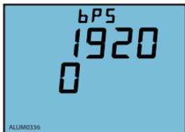
Fig.3-38 Baud rate setting
