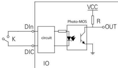
Fig.2-28 DI input circuit diagram
