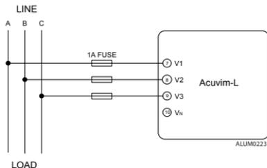
Fig.2-14 3LL 3-phase 3-line direct connection
