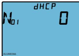
Fig.3-73 PROFIBUS address setting
